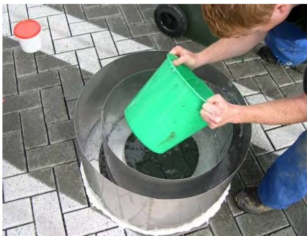
Figure 24: Infiltration Test on Permeable Pavers
