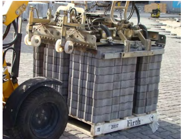
Figure 29: Paver Laying Machine
