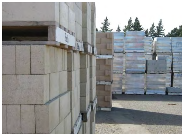
Figure 36: Cubed Pallets of Concrete Blocks
